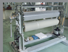
Masroll roll-stand unit with cylinder actuators. All stainless steel structure model.
