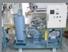
Nash-type vacuum unit, normally for water-related, with an exhaust separator.
